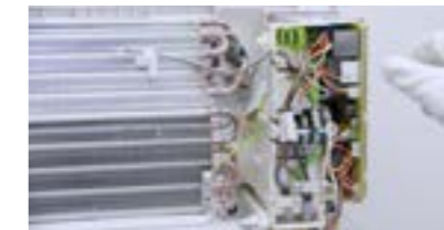
Disconnect all the connectors.
